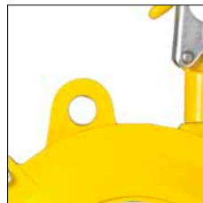
Suspension eye according DIN 15112 spring balancers must be equipped with additional suspension eyes for the attachment of secondary safety chains.
