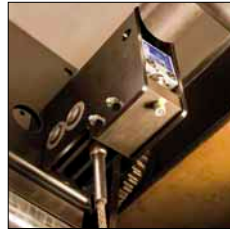
Overload prevention device prevents lifting excessive loads
